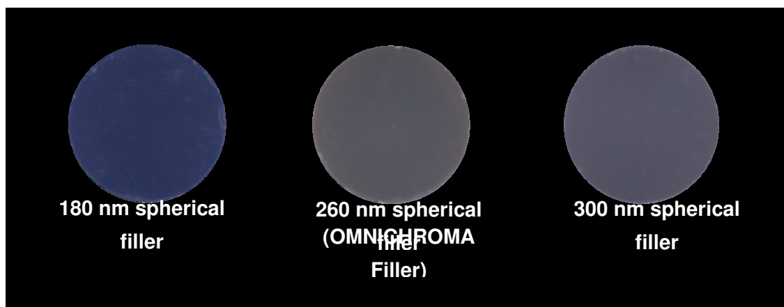
Fig. 10 Color difference of the resin composites consisted of specifically sized spherical fillers on a black background.
