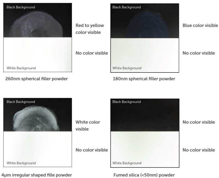
Fig. 9 Relationship between particle size and structural color phenomenon.
